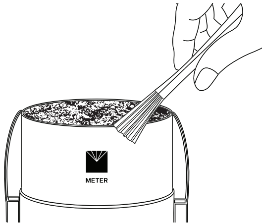
Figure 49 Fix and clean the soil sampling ring
