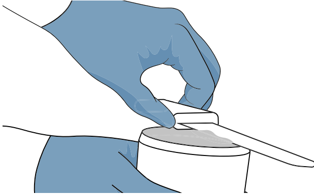
Figure 10 Cut protruding soil on cutting side of sample ring
