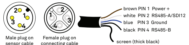
Figure 5 4-pin M12 cable type
